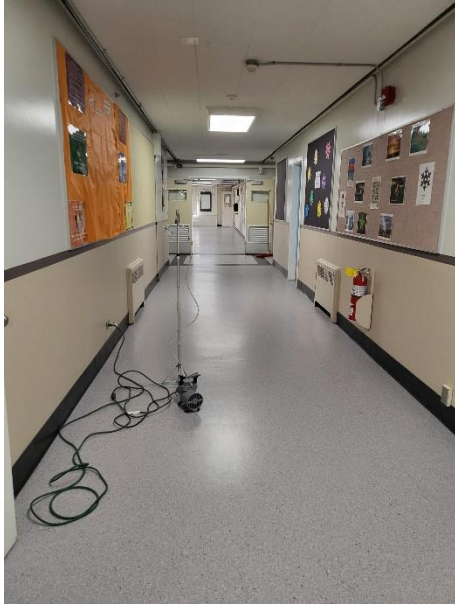
Photo: 1 Sample: 55160-ST1 Location: Playground Entrance - Hall Description: Fungal Spore Trap Sample
