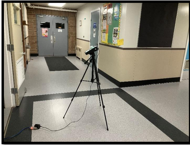
Mould air sample collected within the West Hallway.
