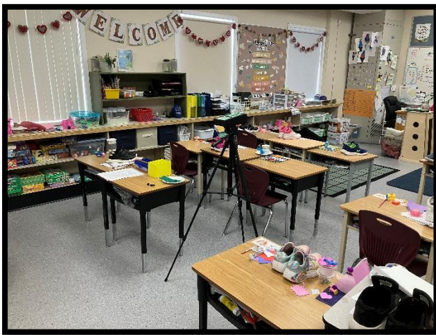
Mould air sample collected within Classroom 21.
