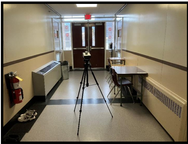
Mould air sample collected within the North End of the North Hallway.
